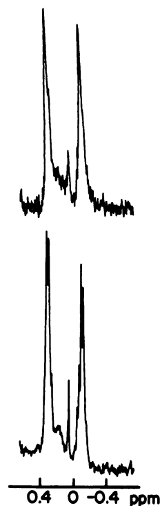
FIG. 6. Signals of the two isopropyl methyls in the 240-MHz NMR spectrum of zinc-complexed isomer II of the AIA adduct
